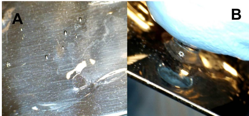
Figure 3: A SS tag sprayed with Prepclean and left bagged for 100 h. the gel retained its moist characteristics.
